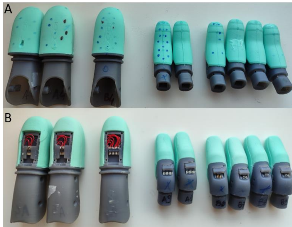
Fig 9. Photos of (a) front and (b) rear side of the as-fabricated Mia hand fingers integrated with e-skin where the blue/black dots mark the position of sensors inside the artificial skin used for electrical measurements.
