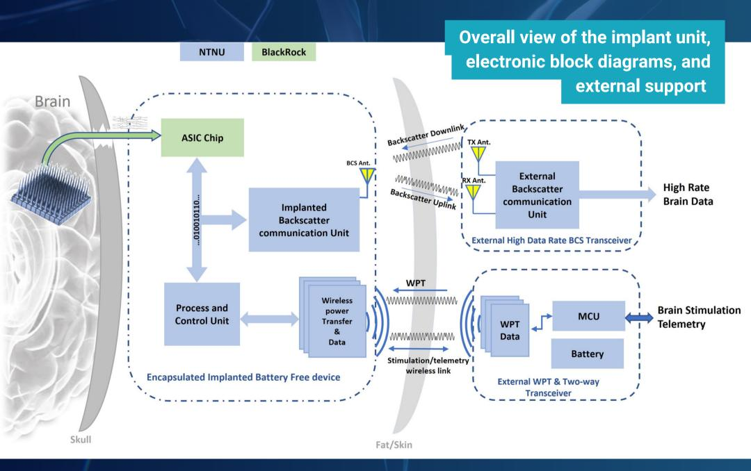
The **external unit** reads implant data using the RF backscattering technique. It includes a **wideband antenna** to support the required bandwidth of the data, a **local RF generator**, **receiver and transmitter chains**.
