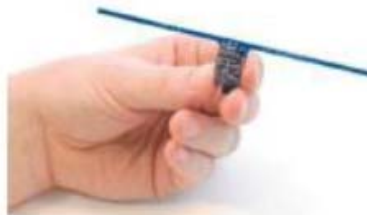
Intel WISP RFID tags harvest energy from RF radiation
