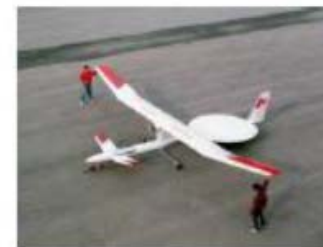
The SHARP unmanned plane receives energy beamed from the ground
