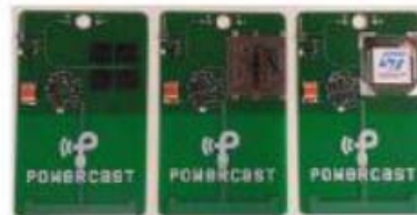
Powercast RF harvesting circuit for sensor networks
